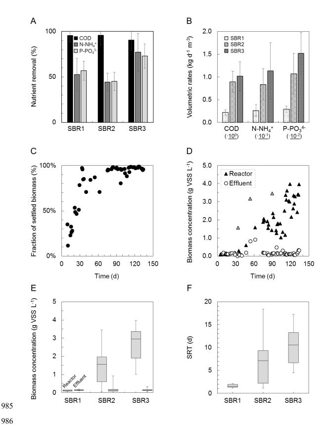
Figure 2. Nutrient removal and biomass characteristics across SBR operations in the mixedculture PNSB photobioreactor. A: Increases in COD, ammonium, and orthophosphate nutrient
