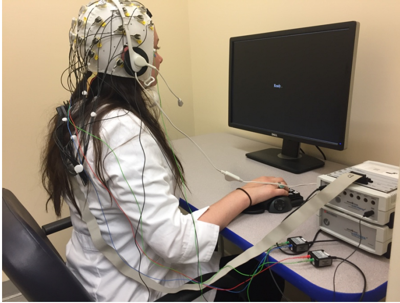
Figure 2. Example of the S-1 Voice Key device used to collect digitized time stamps of response times of cued recall for semantic associates in the current study, concurrent with EEG recordings.
