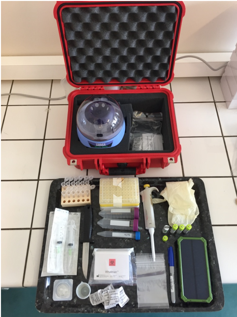
S1 Fig. Portable Laboratory carrying case used for liquid biopsy sampling. The case contains a battery powered minicentrifuge and a portable solar panel battery charger for long term expeditions. The case also contains all necessary reagents and equipment to collect biopsies on site.
