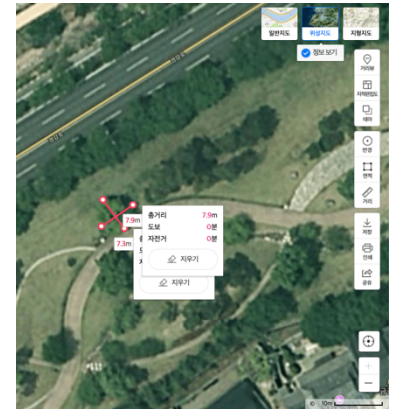
Figure 1. An example of measuring the shortest and the longest crown diameters of a tree.
