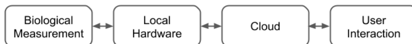
Figure 1. Cloud-based experiment paradigm: biological measurement and local hardware are presented to the user through the cloud, such that experiment management and control can be administrated remotely and may be automated by a computer program.
