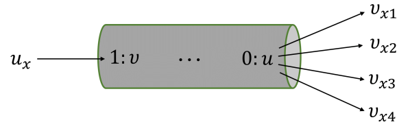
Fig 7. The template bond graph module for intermediate vessels in our version of the ADAN open-loop model. The number of v_x variables depends on the maximum number of branches occurring in any segment. Here, four auxiliary variables corresponding to four branches are demonstrated.
