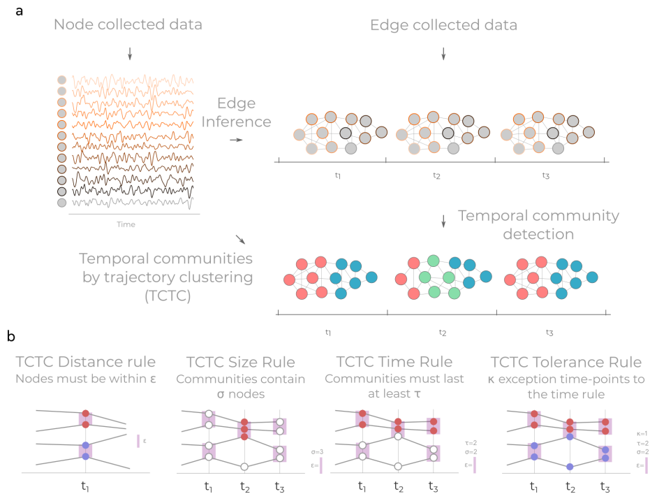
Figure 1: An illustration of TCTC. a How TCTC relates to other methods. Flow chart showing how temporal communities are derived contrasting TCTC from 2-step procedures on node collected data. Temporal communities can be derived on edge collected data in one step, node collected data in two steps via edge inference, and node collected data with TCTC in one step. b The four rules that define trajectories in TCTC. All four rules need to be obeyed in order to define a trajectory. Each rule shows four time-series with one or three discrete time-points. Purple rectangles show instances where the distance rule is successfully applied. White nodes indicate no trajectory is found.
