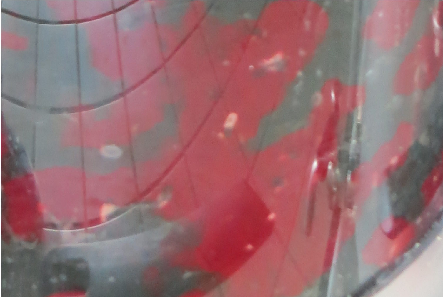
Fig. 1. Photograph of the transparent wall of the anaerobic digester used to analyse the effect of natural sunlight on the microbial community. After three weeks operating de anaerobic digester, a red-pigmented microbial biofilm grew on the inner wall of the reactor forming irregular patches.
