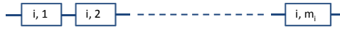
Figure 2: Failure by the i th path at time t requires m_i independent failures to occur in any order, with the last failure at time t (Eq. 5).
