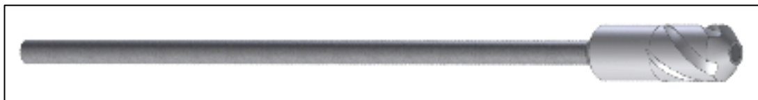
632 Figure 1- Figure Supplement 1: Design of homogenizer used in mini-INTACT
