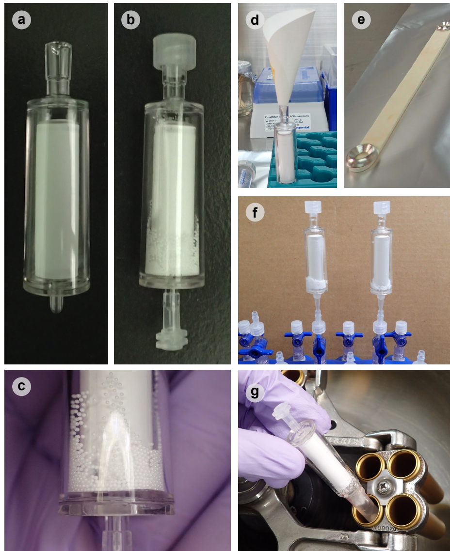
Figure 1: Images of Sterivex TM filter cartridge and zirconia beads. (a) Sterivex cartridge filter without zirconia beads. (b) Sterivex filter cartridge with inlet/outlet caps (inlet, Luer Fitting VRMP6; outlet, Luer Fitting VRSP6). (c) Enlarged image of \phi 0.5 mm zirconia beads. (d) Sterivex TM filter cartridge with a rolled filter paper (ADVANTEC, 5A 90 mm). (e) A hand-made scoop. The scoop is used to add/measure 1 g of zirconia beads. (f) RNAlater solution was removed using QIAvac system (Qiagen, Hilden, Germany) before DNA extraction. (g) The lysate was transferred into a new 2-ml tube from the inlet of the filter cartridge by centrifugation. A capless 2-ml tube was lightly attached by a clean tape to the outlet of the cartridge before the centrifugation.
