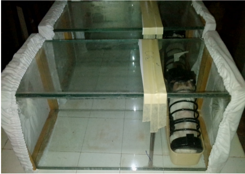
Figure 2: Design for experiments testing host-seeking behavior using guinea pigs and a tunnel choice chamber with nine small holes cut into a barrier between compartments
