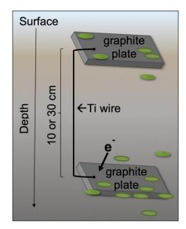
Figure 8. Schematic of an electrodes pair.
