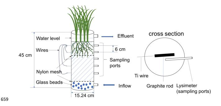
Figure 1. Schematic of a CW mesocosm and electrode setup.
