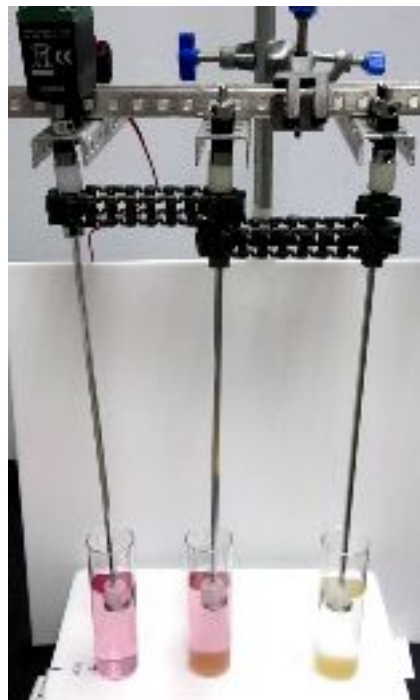
Figure 5. Setup of simulated WWTP tanks. Clear plastic cylinders and rotating central rods that extend into the cylinders mimic water movement in WWTP tanks.
