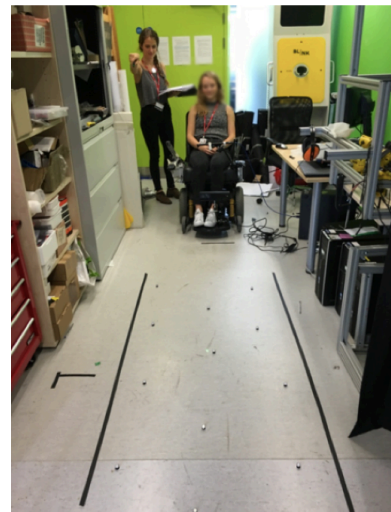
Fig. 3. Test of the 3D Gaze Data Accuracy. The technician is using a laser to indicate 10 different patterns to the user.
