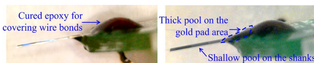
Figure 9. Photos from camera #2 before and after the deionized water application around the epoxy covering the wire bonds between the SSS and PCB.
