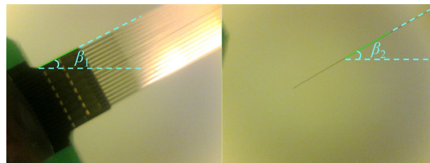
Figure 7. Measurement of shank orientation \beta_1 and CF orientation \beta_2 .
