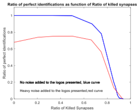
Fig. 5 Ratio of perfect identifications as function of killed neurons when no noise was added to logos (blue curve) and when heavy noise was added to logos (red curve).
