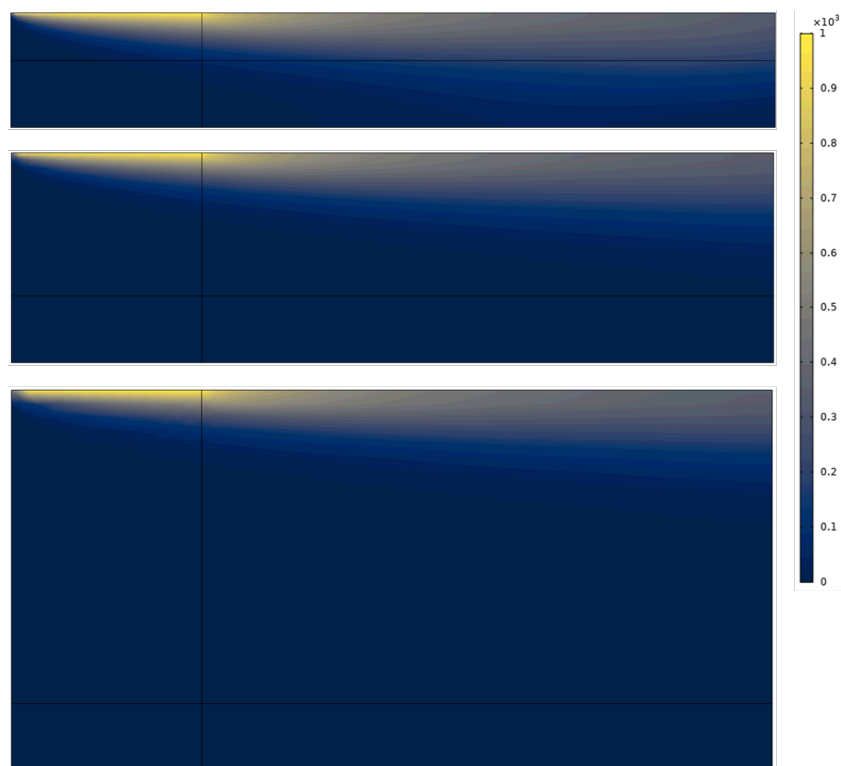
Figure 8: Diffusion profile for a particle with a radius of 20 nm for various mucus depths ( 5\ \mu\text{m} , 15\ \mu\text{m} , and 33\ \mu\text{m} , from top to bottom). Units are in \text{mol}/\text{m}^3 . For a particle of any size, the drug would need to be administered deeper into the lungs than the targeted site to ensure a maximum amount of dosage reaches that area. However, location of the targeted site also determines how much deeper, as less distal lung regions have thicker mucus layers, which take longer to cross.
