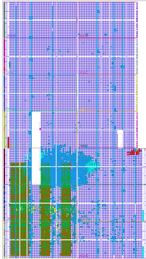
Fig. S12. FPGA resource utilisation. 20% of slice look-up-tables (LUT) for Tapped-delay lines (TDLs) (dark red) and thermomemer-to-binary encoders (T2B) in green; FIFO (98 % of inbuilt BRAM) and 5% of LUT for FX3 module in light-blue; Integrated logic analyzer (ILA) debugger in yellow; SYLAP (only for test purpose) in red - 2% LUT.
