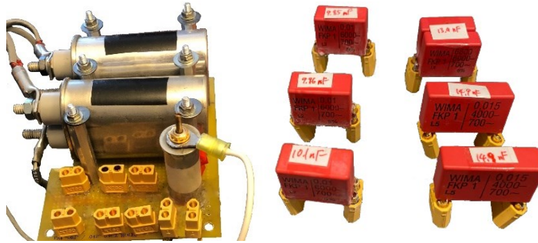
Figure 2. Capacitor bank of the system. Left: capacitor board with sockets (yellow) for interchanging the resonance capacitors for Ch 2 and Ch 3 and the variable capacitor (grey cylinder) for Ch 3. Center: capacitors on quick-change sockets for adjusting the resonance frequency of Ch 2 and Ch 3. Right: Layout of the Litz wires within the cable, with the interference shielding as the outer-most layer.
