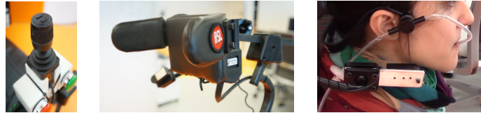
Figure 1: Control interfaces used in the study. From left to right: 3-axis joystick, head array device, sip/puff switch.
