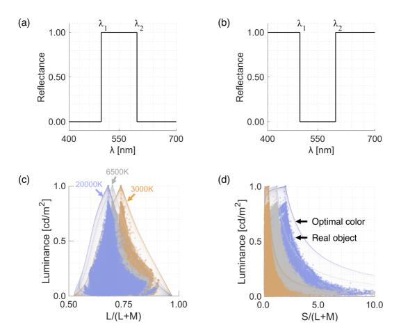
Figure 1: (a), (b) An example of band-pass and band-stop optimal color. (c), (d) Chromaticity versus luminance distributions of 102,721 optimal colors and 49,667 real objects under illuminants of 3000K, 6500K and 20000K.
