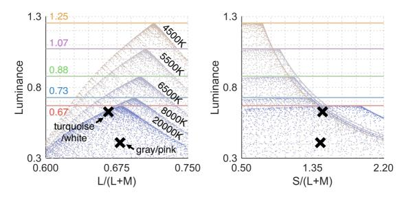
Figure 5: Best-fit optimal color distributions at different intensity levels. We see that estimated color temperature continuously changes from high to low color temperature as the estimated illuminant intensity increases.
