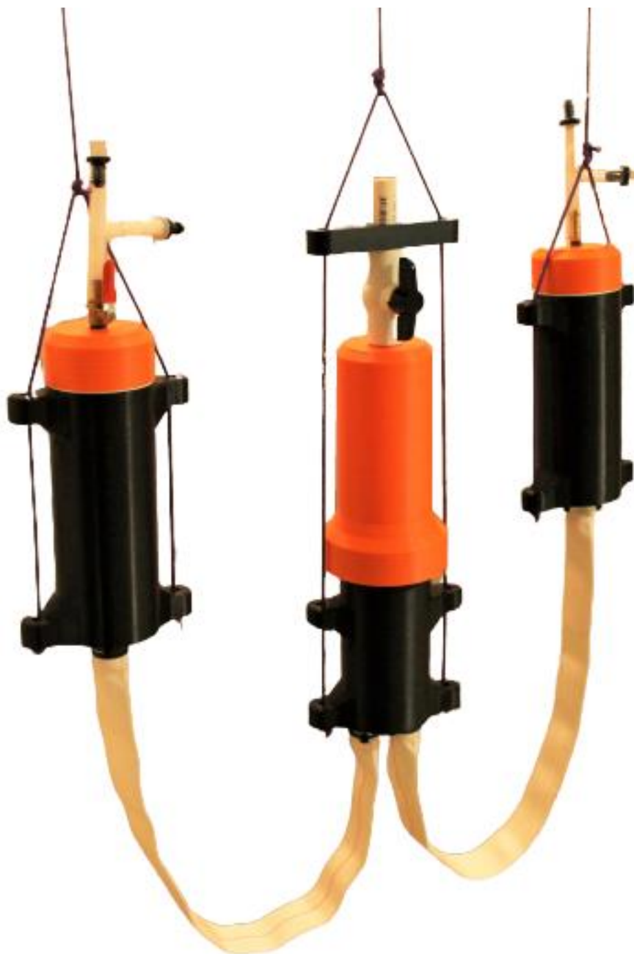
Fig. 6. 3D printed ventilator assembled prior to testing pressure and ventilation rate
