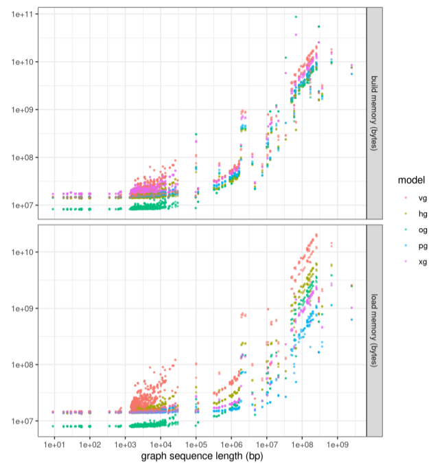
Fig. 3. Memory requirements for model construction and loading. Memory costs versus graph sequence size for the graph collection, colored by HandleGraph model. The memory requirements for graph construction tend to be higher than those for loading the graph model. All methods show fixed overheads of several megabytes, seen in the flat tail to the left of both plots. Outside of this region, all methods show roughly linear scaling in both build and load costs per input base pair. The relative differences in memory costs appear to be stable between different methods across many orders of magnitude in graph size. Notably, vg has approximately the same build and load costs, as the data structures used are the same. The other methods tend to use auxiliary data structures at build time, and so require more memory to build the data structure than to load it.
