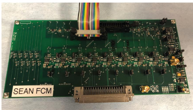
Supplemental Figure 3. Block diagram of the measurement electronics and photograph of the PCB. The GMR sensors are modulated by a sinusoidal voltage and the resulting currents are quantized by a transimpedance amplifier (TIA) and an ADC. A bleed resistor ( R_B ) removes most of the sensor baseline current. Digital signal processing performs demodulation then applies matched filtering and cross correlation to enable high SNR signal detection.
