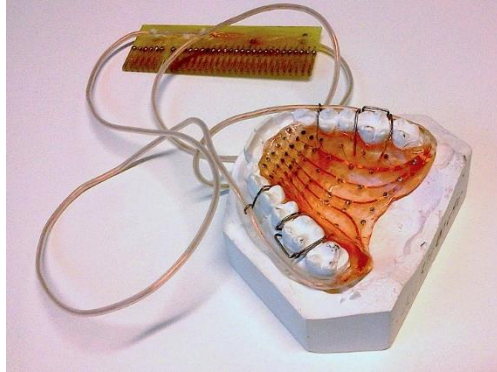
Fig. 1. An electropalate mounted on a stone cast of a human palate. The figure shows the stone cast in white, with the palate and its electrodes mounted on the cast. Wires connect the electrodes to an external interface which is connected to a computer to read the signals from the electropalate.
