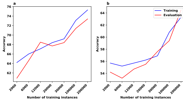
Figure 6: The training and evaluation accuracy in the noise_inference problem for SVM. All matrices for this experiment are of size 10 \times 10 and are column-sorted. The x-axis corresponds to the training sample size. (a) Training and evaluation accuracy for \alpha = 0.002 and \beta = 0.1 (for the noisy matrices). (b) Training and evaluation accuracy for \alpha = 4 \times 10^{-4} and \beta = 0.02 (for the noisy matrices).
