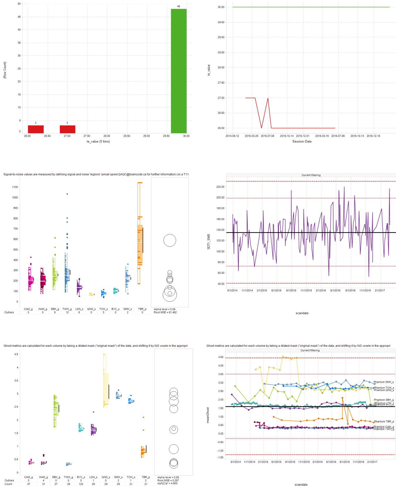
Figure 4: Sample images from the MR Quality Assurance (QA) and Control (QC) Spotfire dashboards. Top panel: Cross-sectional (left) and longitudinal (right) displays of the Scan Acquisition Parameter QA Dashboard depicting the Resting State fMRI TE values acquired from 54 scans from one ONDRI site. Green and red traces represent scans that were within and outside of the expected range, respectively. Middle panel: Cross-sectional display (left) of the Structural QC Pipeline Dashboard depicting signal-to-noise ratio (SNR) results of 3DT1 scans obtained at each of the ONDRI sites. Right panel depicts the longitudinal display of the same results for one site. Dashed and dotted horizontal red lines indicating \pm 3 and 2 standard deviation limits, respectively, of the site's overall SNR average. Bottom panel: Cross-sectional (left) display of the fBIRN Phantom QA Results Dashboard depicting the 'Ghosting value' results from the monthly Resting State fMRI scans of the fBIRN phantom. Right panel depicts the longitudinal display of those results from each of the ONDRI scanners (separate lines), with dashed and dotted horizontal red lines indicating \pm 3 and 2 standard deviation limits, respectively, of the overall datapoint values.
