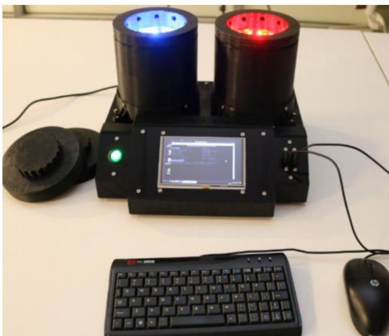
Figure 10: Fabricated optical stimulator. The prototype was fabricated, tested and employed to assess blue-light induced retinal degeneration in Drosophila flies.
