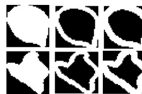
Figure 6: Trimap visualization on the DDSM-BCRP dataset. Images in the first column are the segmentation groundtruth. Images in the second column are the trimaps of width 2. Images in the third column are the trimaps of width 3.
