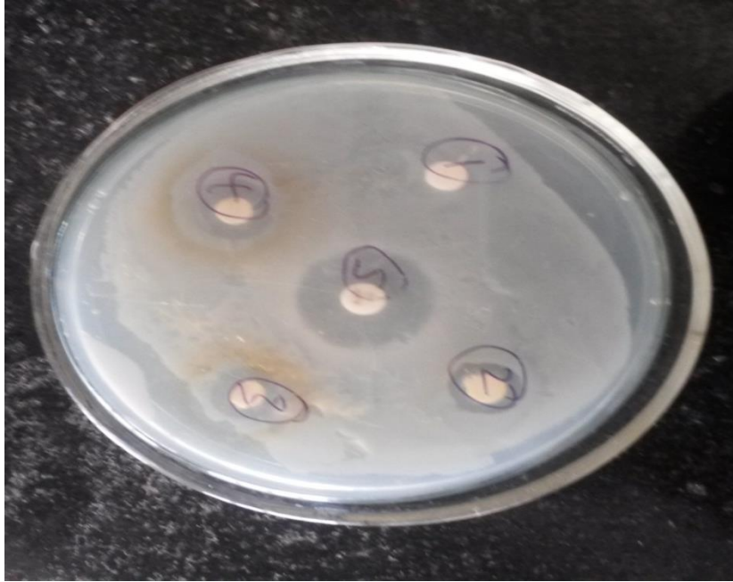
Fig 4.2.1b: Treatment 1: Isopropanol ; Treatment 2:0.02g of copper/ml of titanium isopropoxide; Treatment 3:0.04g of copper/ml of titanium isopropoxide; Treatment 4:0.06g of copper/ml of titanium isopropoxide; standard.
