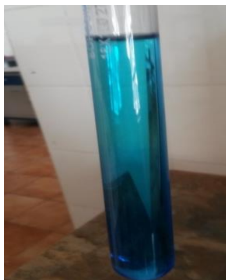
Fig 4.2.3: Methylene blue reduction test of water: a) Methylene blue with E.coli and b) Methylene blue with E.coli and TiO 2 .
