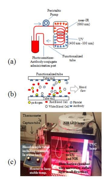
Fig. 1. (a) Schematic of the set-up. (b) Capturing by antibody immobilization on tube. (c) Experimental setting of the system. The tubes that are exposed to UV and NIR along with the light sources are placed inside a mirror chamber. One side of the chamber was opened for this picture. The entire set-up resided inside a biosafety cabinet.
