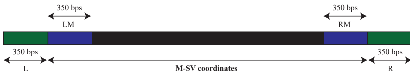
Figure 1: Annotations are generated for each SV for five different regions in and around the SV: Left flanking region (L), Left middle flanking region (LM), Middle regions based on SV coordinates (M), Right middle flanking region (RM), and Right flanking region (R).
