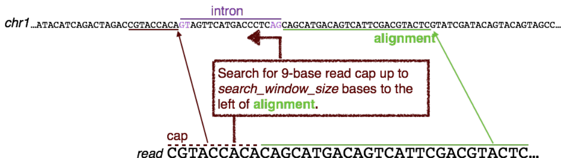
Figure 10: Rail-RNA searches for a match to the read cap that overlaps no aligned readlets if the cap spans at least min_exon_size bases, where min_exon_size is by default 9.
