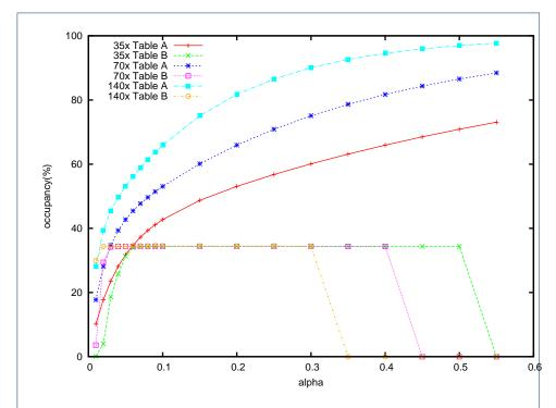
Figure 4 The effect of  $\alpha$  on occupancy of Bloom filters A and B The effect of  $\alpha$  on occupancy of Bloom filters A and B using simulated  $35\times$ ,  $70\times$  and  $140\times$  datasets. The error rate is 1%
