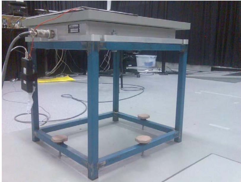
393 Figure 1: Forceplate fixed to a frame to provide a stepping platform for the repetitive stepping 394 task. Note the pressure switch on the top of the platform with battery pack attached with red 395 wire (left side of frame)
