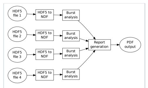
**Figure 5** Example of the CARMEN workflow facility. Ellipses denote files and boxes denote CARMEN services. Four HDF5 files are independently converted into NDF for burst analysis. The outputs (in this case, the duration of each burst detected on each electrode) are then collated into a report generation service to produce a graphical summary, shown in Figure 6. (Static)
