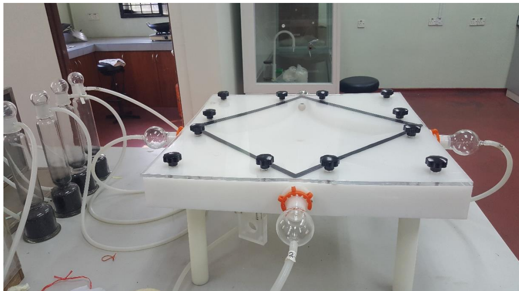
Fig. 1. Four arm olfactometer with glass flask at the end of each arm.
